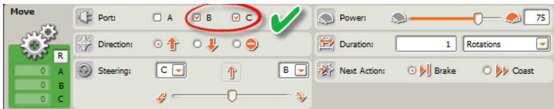
Figure 4.31: NXT configuration panel with matching ports for move block.
